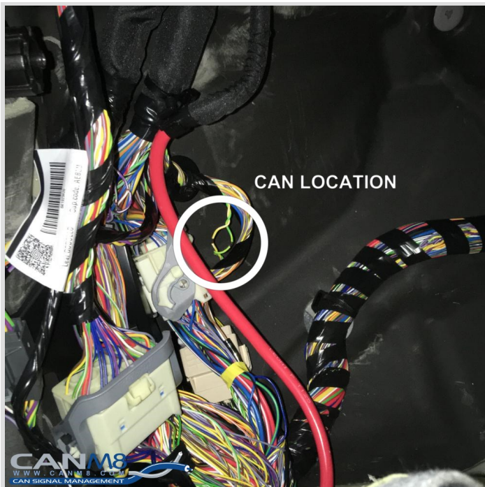
Wiring harness containing the Headlamp CAN
