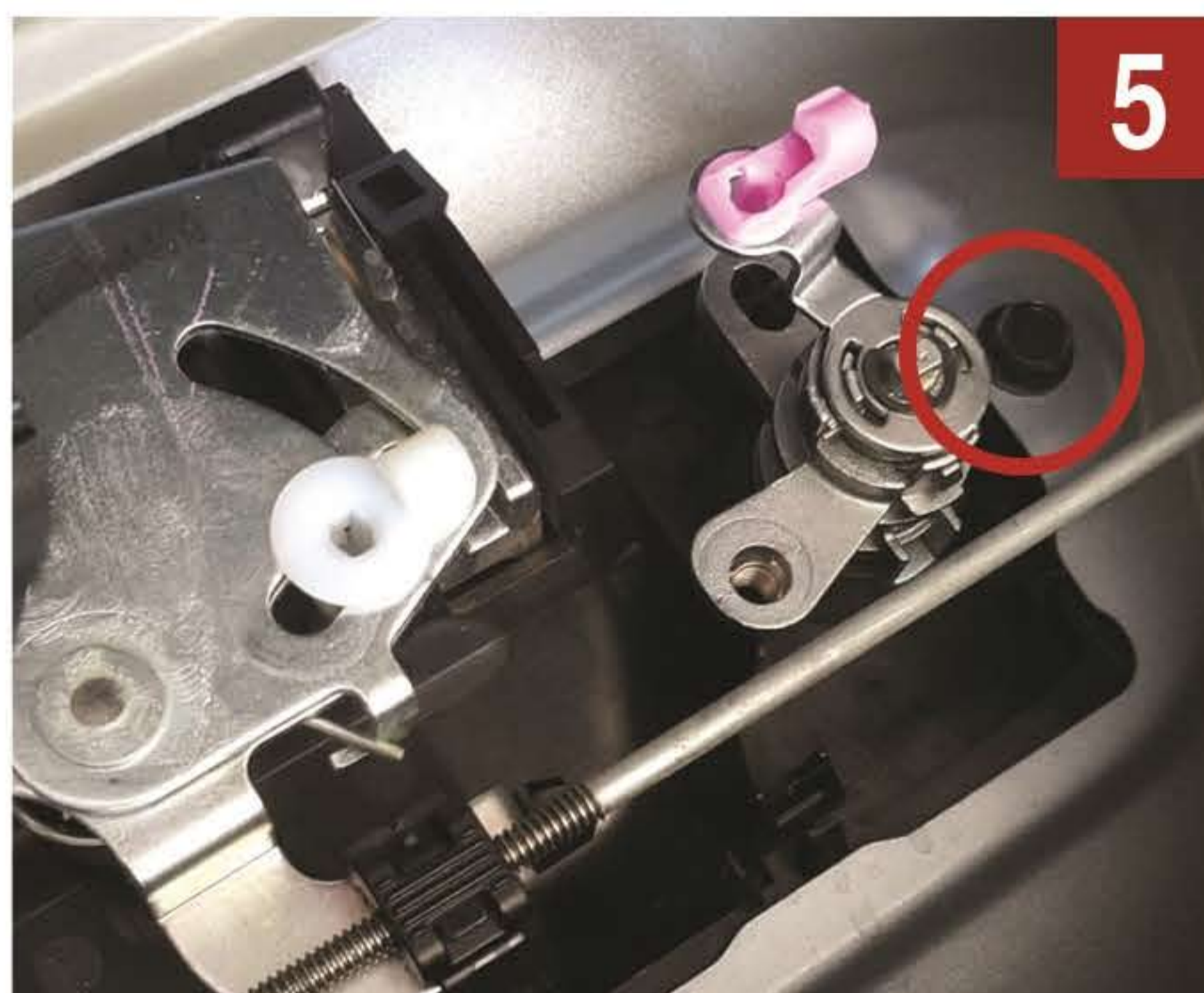
5 REMOVE SHEAR BOLTS WITH SOCKET WRENCH
