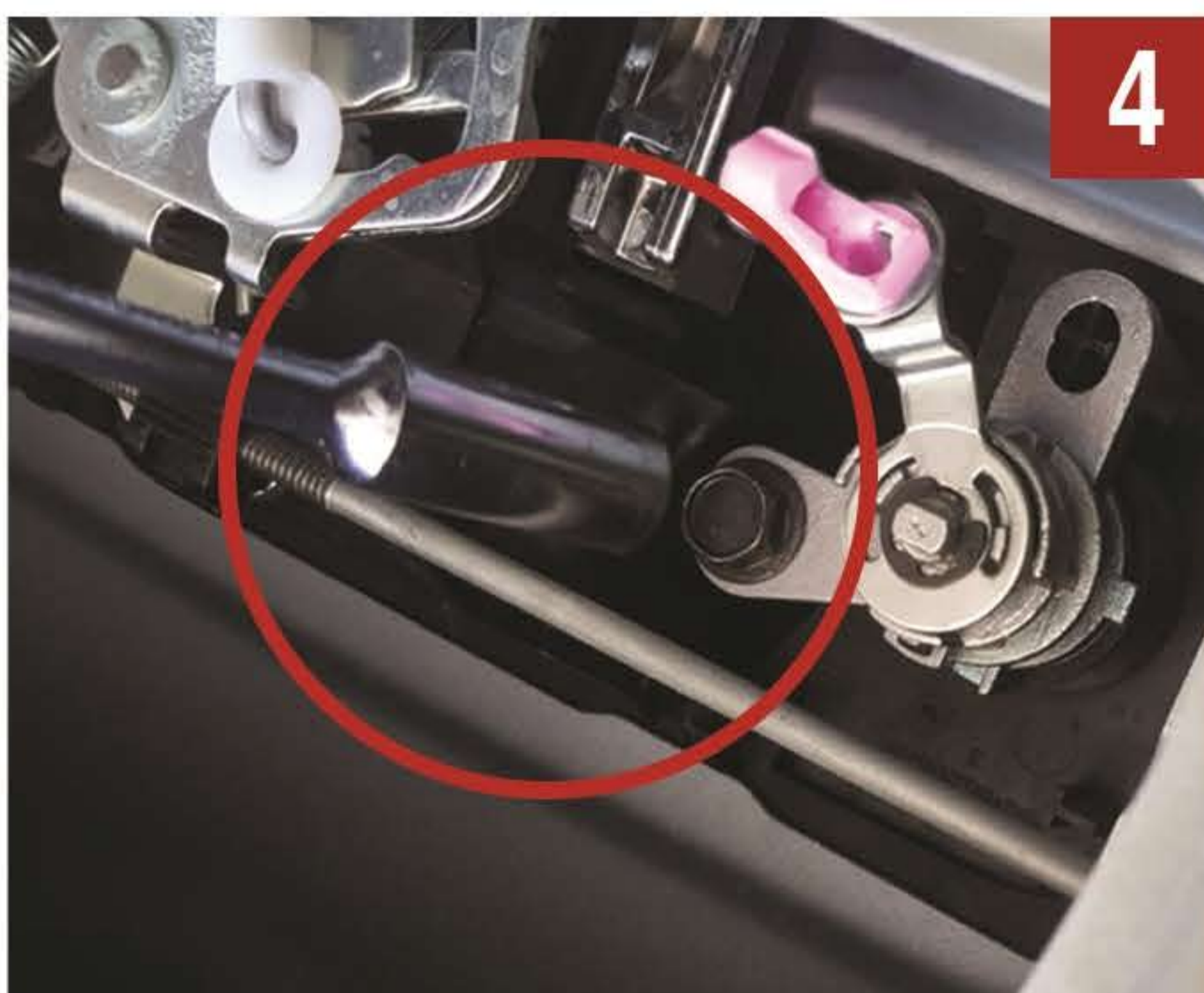
4 REMOVE SHEAR BOLTS WITH SOCKET WRENCH
